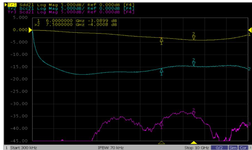
SCM201212HDMITL-670 Insertion Loss Curve
